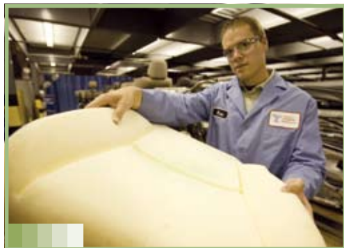
Toyota is using a renewable resource — soybeans — in the foam of passenger seats in the Toyota Corolla and the Lexus RX.
