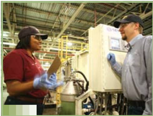
At our plant in Alabama, employees from the environmental department worked with production to implement a coolant recycling process.
