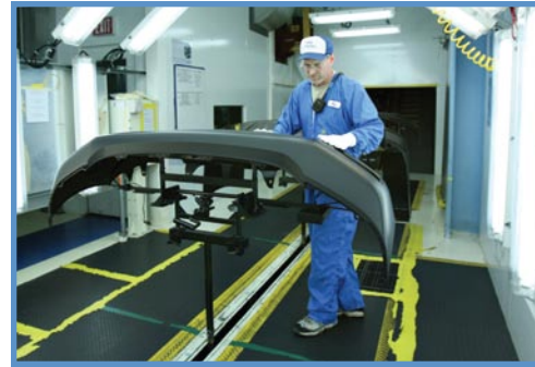
An employee at our plant in Indiana inspects a bumper that has just been painted with a water-based primer.
