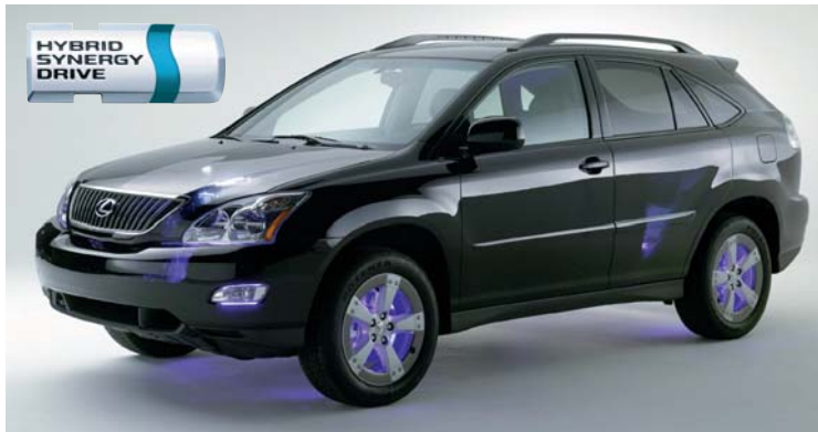
This photo composite illustrates the placement of some of the Hybrid Synergy Drive components in an all-wheel drive Lexus RX 330. A V6 engine and electric motor are under the hood; another electric motor powers the rear wheels.
