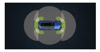
**ADVANCED PARK** uses information from the vehicle's sensors to measure parking spaces and detect objects around the vehicle.
