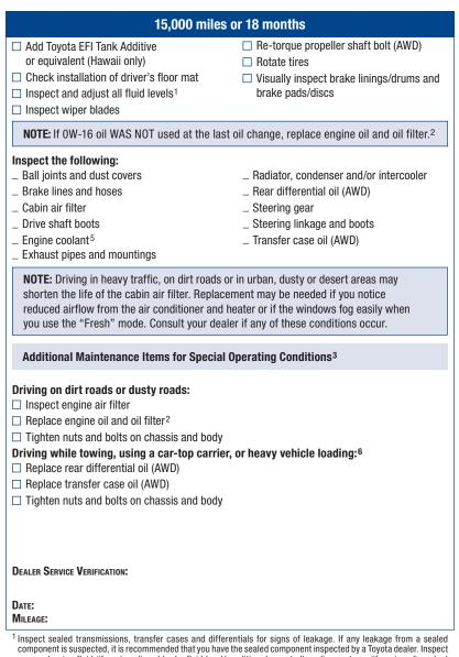
component is suspected, it is recommended that you have the sealed component inspected by a Toyota dealer. Inspect power steering fluid (if equipped) and brake fluid level/condition. Inspect all cooling systems (if equipped) coolant level/condition/freezing point. Your dealer may recommend services (Dealer-Recommended Maintenance) based on inspection results.
