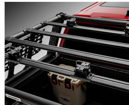
**Go Rhino<sup>®</sup> Quick Release Rooftop Tent Bracket Kit** is designed to work with 4-CORE slotted cross bars and feature an easy pull-pin release, allowing for quick tent removal and easy storage.
