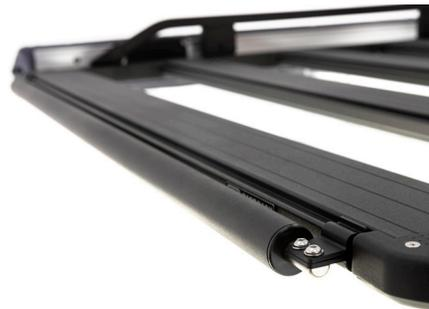
**ARB Base Rack Roller Kit** helps with loading long pieces of timber and other heavy items by adding a roller to the end of your Base Rack. Requires ARB Base Rack.
