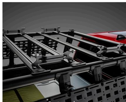
**Go Rhino<sup>®</sup> XRS to SRM Connector Kit** makes mounting SRM basket racks to XRS Xtreme racks quick and easy.
