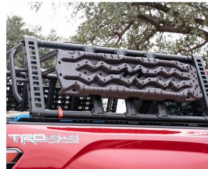
**ARB TRED (Total Recovery & Extraction Device) Pro Grey** is an effective recovery device designed to help get you out of trouble when traction is lost in tough conditions such as sand, mud, or snow.
