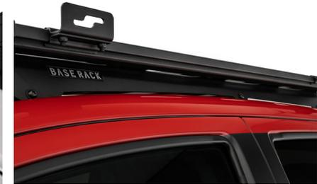
**ARB Quick Release Awning Brackets** provide excellent mounting options for ARB Awnings to ARB roof racks. Requires ARB Base Rack.
