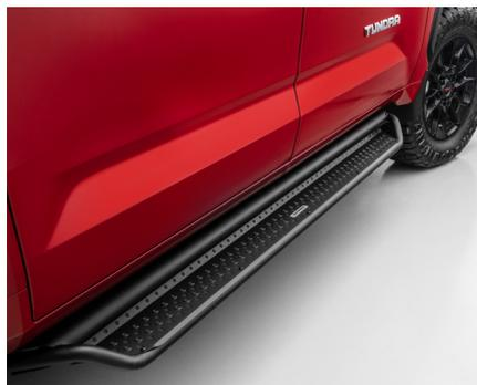
**Go Rhino<sup>®</sup> Dominator Xtreme D1 Running Boards** with full-length drop down steps and a full-length slider design on the bottom surface.
