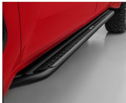
**Go Rhino<sup>®</sup> Dominator XTREME DSS Slider Running Boards** feature a rub rail and an optional full-length step and full-length slider design on the bottom surface.
