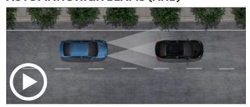
AHB<sup>4</sup> is a safety system designed to help the driver see more clearly at night – while reducing glare for other drivers. By using high beams more frequently, the system may allow for earlier detection of pedestrians and obstacles.
