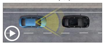
PCS<sup>2</sup> is an integrated camera and laser system designed to help mitigate or avoid a potential frontal collision\*. For 2019 model year vehicles, TSS-C's PCS has been enhanced with the addition of pedestrian detection.
