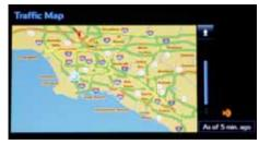
The Traffic App displays a scrollable map showing local traffic in 3 colors. Traffic conditions are displayed in red, yellow and green for heavy, moderate or light traffic conditions. Use  $\blacksquare$  arrows to scroll the map up or down.
