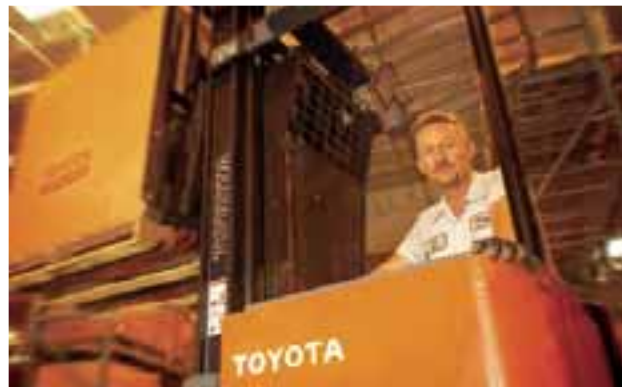
Our Los Angeles parts distribution center replaced approximately 300 gallons of hydraulic fluid with vegetable oil in trash compactors and forklifts. Here, associate Johnny Haire is seen driving one of these forklifts.
