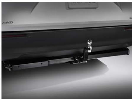
Towing hitch receiver and wiring harness<sup>50,51</sup>
